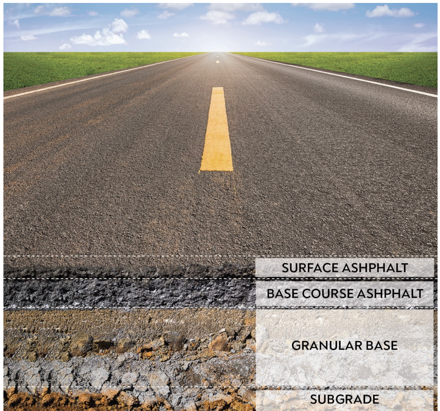
Fig. 3.8 Cross-section of a road segment.
